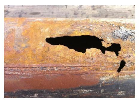
Figure 8. Corroded tail gas line
