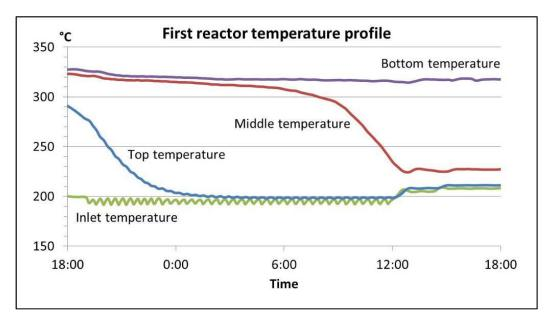
Fig. 19 shows that a select set of data can show you what is happening in the SRU.
