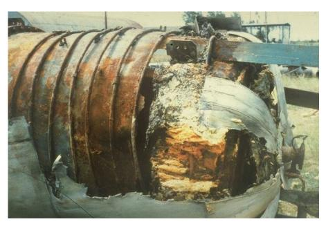
Figure 15. Coalescer damaged by sulphur fire
