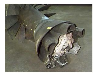
Figure 2. Burner throat damaged by backfiring
