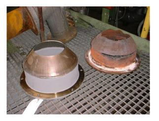
Figure 3. Undamaged and damaged burner throat
