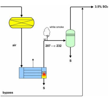
Figure 14. Sulphur fire in final condenser
