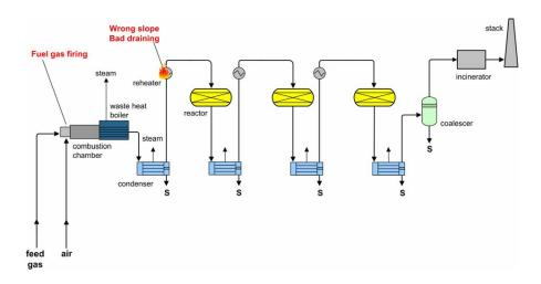
Figure 11. Sulphur fire at the first reheater Case
