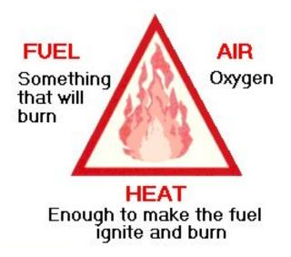
Figure 10. Conditions for a sulphur fire
