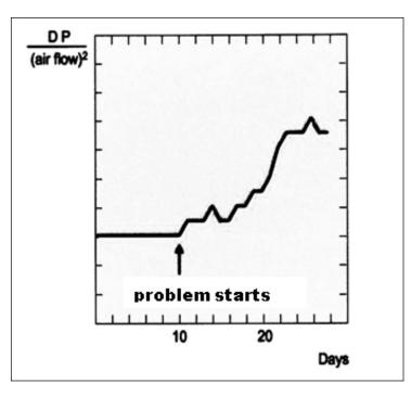
Figure 17. Monitoring pressure drop
