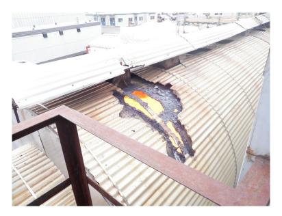
Figure 4. Damaged shell after refractory failure
