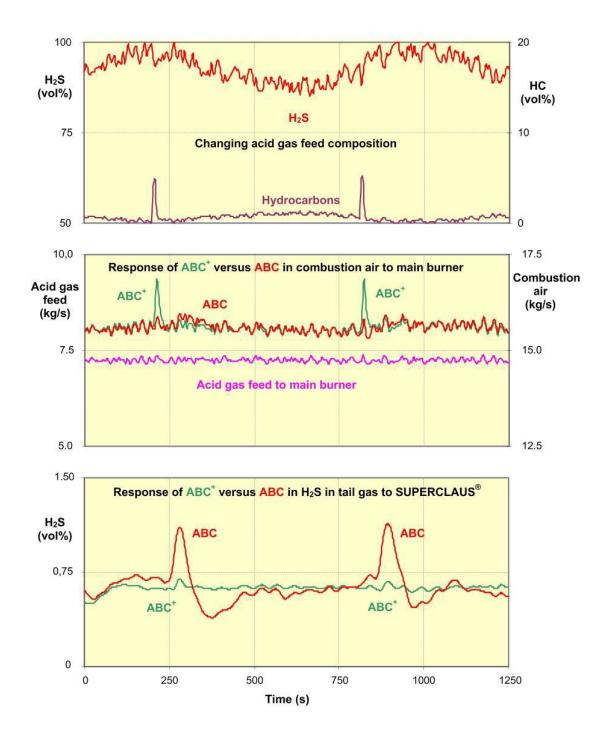
Figure 7. Improved burner control response using ABC+
